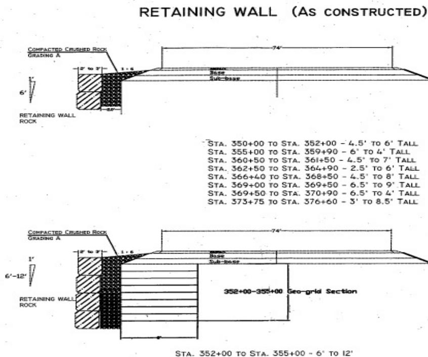
Appeal File at 653. The construction method of blocks of rock and compacted rock was used in the construction. In contrast, work which required the use of a geogrid, a different construction method, is depicted with a different as-built diagram and was treated as a change within the scope of the contract. Appeal File at 653.
